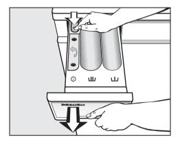
The pre-wash and main wash compartments of the detergent drawer are self-cleaning. However, for hygiene reasons the entire detergent drawer should be cleaned as follows on a regular basis.
